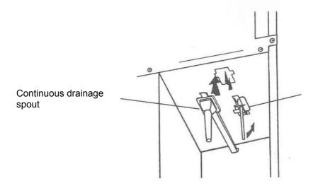
Container full cutout microswitch depressed when spout for continuous drainage is fitted.
