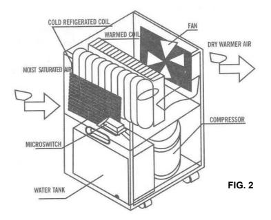
Your dehumidifier controls humidity by forcing excess moisture to condense from the air into the unit as it passes over the cooling elements. Contact with this cold surface causes the moisture in the air to condense. This condensed water then drains safely into the water tank. The dried air then passes through a warmed coil where it slightly warmed and re-enters the room at a slightly elevated temperature.
